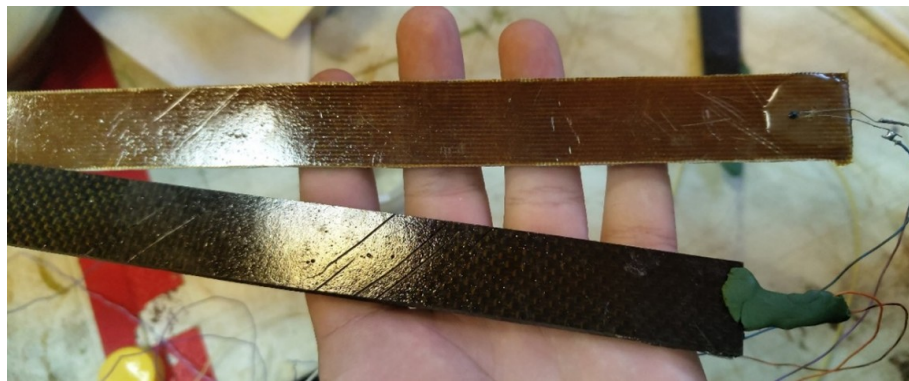
Fig. 5. Samples with a fixed thermistor: fiberglass (top) and carbon (bottom).
