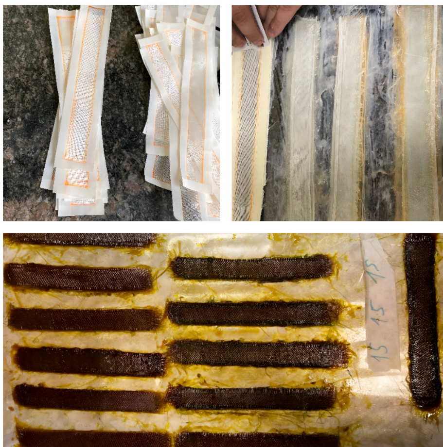
Fig. 1. Process of sample manufacturing: fiber cutting (top left), impregnation and removing of resin (top right), drying of samples (bottom).
